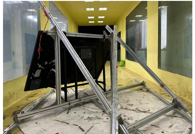
1# Rear Wind direction angle:135° installation inclination: 35°
