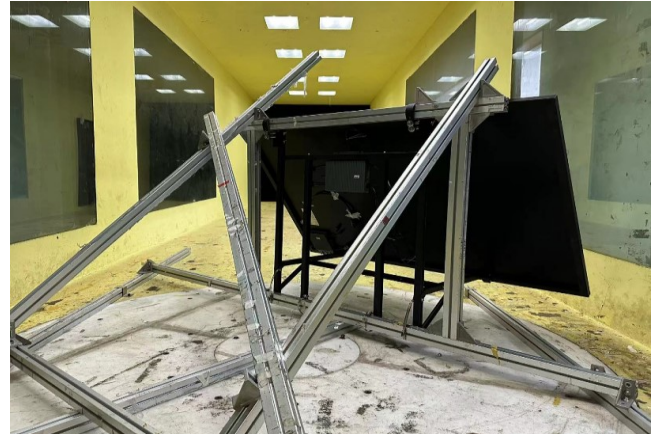
1# Rear Wind direction angle 45° installation inclination: 35°
